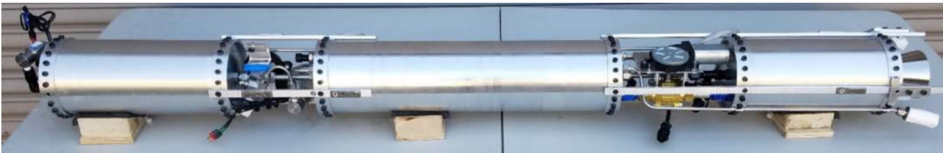
◀ Spitfire liquid rocket engine stack, 2018
